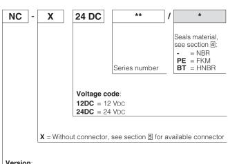
${f NC}\!=\!{\sf normally}$  closed in rest position NO=normally open in rest position
